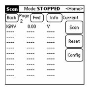
The second page is configured for just ignition voltage. This can be useful to determine the state of health of your battery. Turn the key on, start scanning this page, then start the car. Then click the "Info" button to see the minimum voltage that occurred while cranking the engine over. If it's less than 9.5V, your battery may be on its way out.
